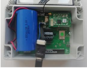
The LoRaWAN Board (left image) can be powered by the config adapter. Other devices, like the NB-IoT /LTE-M boards or the wMBus LoRaWAN Bridge V2, need to be connected to their normal power supply. If in doubt, just make sure you have the device powered!
