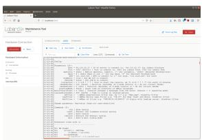
All of our Devices provide extensive logging information over the *CONFIG* port. When you are connected to a Device in the Lobaro Maintenance Tool, you can read the log messages in the *LOGS* Tab. This feature is helpful if you try to find out the cause of problems you experience. You can also find out a lot of information about your Device, for example you can find the parameters used to connect your LoRaWAN Devices to your Network Server (DevEUI, AppKey, etc.).
