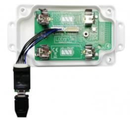
The USB adapter uses a six-wire JST-ZH series connector for attaching to Lobaro hardware at the config connector.
