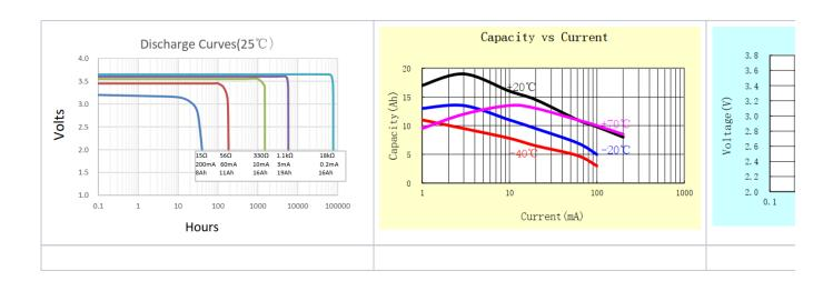
A reasonable alarm value for "Low Voltage" is around 3.2V - some devices might work on lower voltages.
